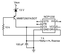
**Figure 2. Overvoltage Protection Circuit**
