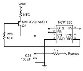
Figure 3. Overtemperature Protection Circuit
