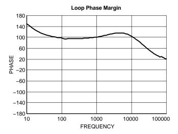
Figure 5. Excel Spreadsheet Phase Margin
