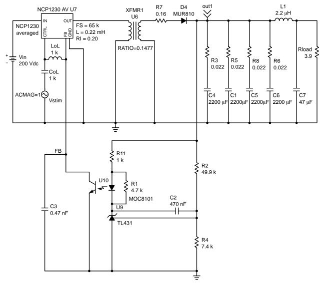
Figure 7. AC Frequency Response SPICE Model
